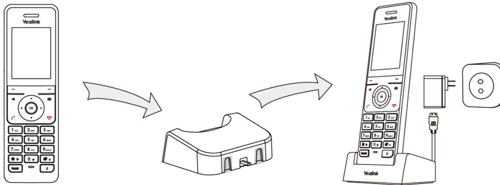
**Note** The handset should be used with Yealink original power adapter (5V/600mA) only. The use of the third-party power adapter may cause the damage to the handset.
